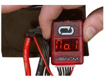
After the battery is fully charged use the supplied voltage meter to check that each cell in the battery is within 0.1 volts of each other. At full charge each cell will be around 4.2 volts. If the cells have a difference in voltage greater than 0.1 volts, that battery should be taken out of service. The voltage meter display will cycle through the cell number, then cell voltage. After cycling through each cell it will display ALL then the total voltage.
