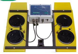
The AutoNav is now wired into the HyDrone and ready for optional equipment.
