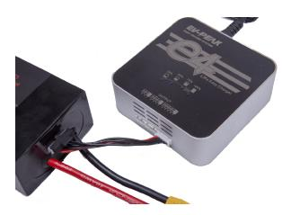
Plug balance cord into the right most port on the EV-Peak charge labeled, OUTPUT [4S|3S|2S|1S|-]
