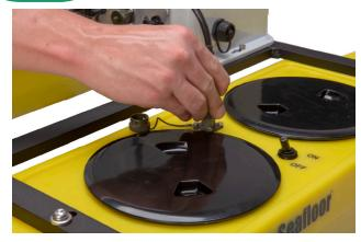
Plug the corresponding PORT and STBD cords from the AutoNav into each of the pontoons.
