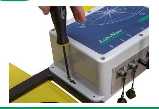
The HyDrone frame is pre-drilled and tapped for the AutoNav. Use the  $^{10}/_{32}$  x  $1^{1}/_{4}$  stainless steel hardware and the provided  $^{5}/_{32}$  allen key to secure the AutoNav to HyDrone frame.
