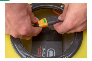
Plug the 14.8 (4S) battery in to the Hy-Drone with the XT90 plug.
