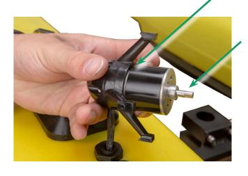
Most importantly clean the area between the motor assembly and the thruster base as well as the gap, as long grass, fishing line, anything thin and long will end up in there. A paperclip or small Allen key works for cleaning it out..
