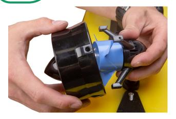
Pull the base and propeller out of the nozzle and tail cone.
