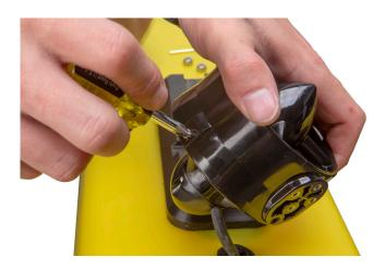
Remove the four #2 Phillips screws along the outer edge of the thruster.
