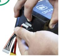
Install balance cords on the batteries that will be charged.
