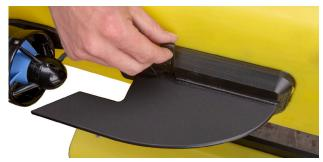
Turn the HyDrone upside down or leaned onto one side gain access to the bottom of the HyDrone. Then slide the fins into the fin mount channel that are in front of the thrusters. Make sure to slide the fin locking pin into the side of the fin mount to secure the fins in place.
