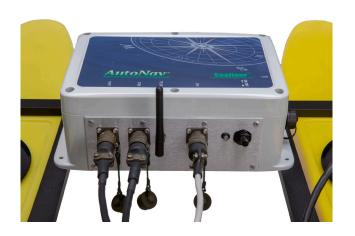
Plug the GPS into the GPS port on the AutoNav.
