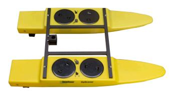
Place the HyDrone frame across the top of both pontoons. Loosely attach the pontoons to the frame with the  $^{1}/_{4}$  - 20x1 stainless steel hardware. Once the four bolts are installed tighten them with the provided  $^{5}/_{32}$  allen key.
