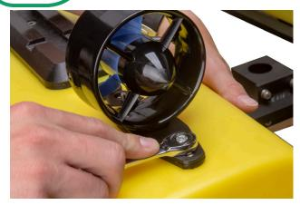
With 3/8<sup>th</sup> or 10mm socket or end wrench remove the nuts on thruster plate that are on either side of the thruster.
