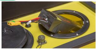
Slide the 14.8 (4S) battery into the hull of the HyDrone with the cords toward stern. Make sure the battery is fully seated into the battery slot.
