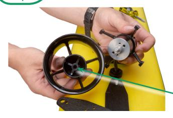
Make sure to clean inside of the nozzle and tail cone.
