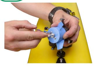
Remove the 2mm allen screw that holds the propeller to the motor assembly.
