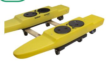
Prepare a raised surface to set the HyDrone pontoons on top of so all the pontoons sit level and the thrusters do not hit the ground. Raised surface should allow the HyDrone pontoons to sit off of the ground roughly 4 inches (150mm) and allow the two pontoons to be roughly one foot (475mm) apart. Remove the Port and Starboard pontoons from the case and set on top of prepared surface.
