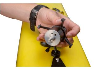
Remove the propeller from motor assembly by putting press on motor shaft while pushing the propeller off of the the motor assembly. Be careful not to put too much pressure on the propeller fins. No further disassembly is required.
