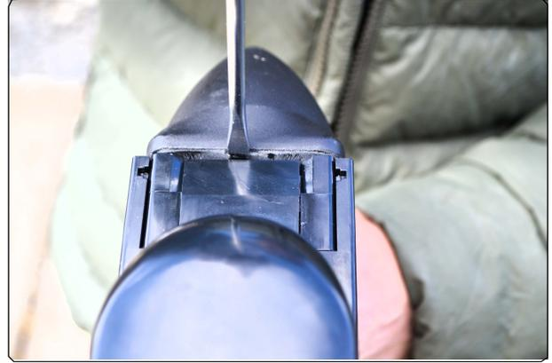
Use pry tool or flathead screwdriver to pop off sides and bottom connectors.
