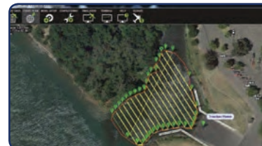
Preplanned survey using Mission Planner
