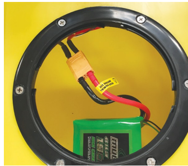
Figure 7—Front access hatch: the battery compartment includes keyed connectors
