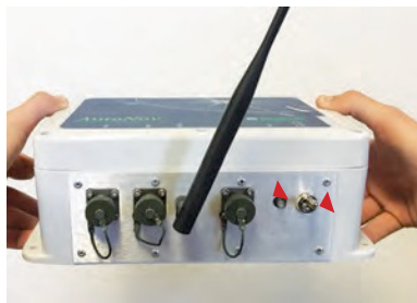
Figure 4: AutoNav On switch on front panel of AutoNav. Red solid and flashin LED on front panel.
