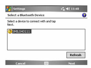
The controller searches for other Bluetooth devices within range. Once the scan is complete, highlight the Bluetooth device to connect to: On a Trimble Tablet tap [Next].
