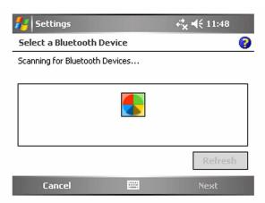
Start a scan on the controller. On a Trimble Tablet, Tap [Add a device]. On a TSC2 controller, tap the [devices] tab and tap. [New Partnership...]. On a Trimble CU (Model 3) controller, tap the [scan device] tab and then tap [scan]. On a Trimble CU controller, tap [Scan Device]. (Do not use [stop] - wait for the scan to complete).
