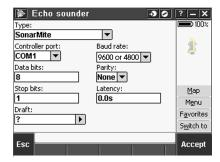
Latency and draft are normally left at 0. The latency caters for echo sounders where the depth is received by the controller after the position. General survey software uses the latency to match and store the depth when it is received with continuous topo points that were saved previously. Tap accept and then tap Store to save changes.
