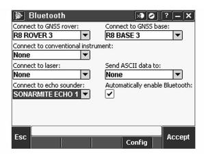
Tap Config and make sure that Bluetooth is switched on. On a TSC2 controller, make sure that the [turn on Bluetooth] and [Make this device discoverable to other devices] check boxes are selected. On a Trimble CU (model 3) controller, select the power tab and then make sure that the [enable bluetooth] and [Discoverable] check boxes are selected. On a Trimble CU controller, make sure that the [Enable Bluetooth] checkbox is selected.
