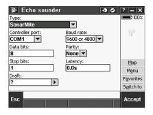
Configure the Controller port: If you set the Controller port to Bluetooth, you must configure the Echosounder bluetooth settings. If you set the Controller port to COM 1 or COM 2, you must configure the port settings.
