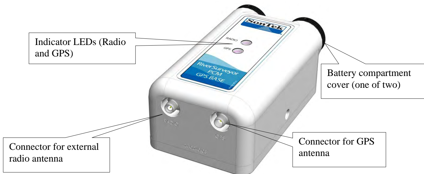
Figure 198. Configuration C – PCM RTK-GPS (Base). The Figure shows the RTK Base Stations and its components.
