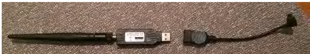
Figure 203. Connecting MicroUSB to USB adapter to SonTek Radio Dongle
