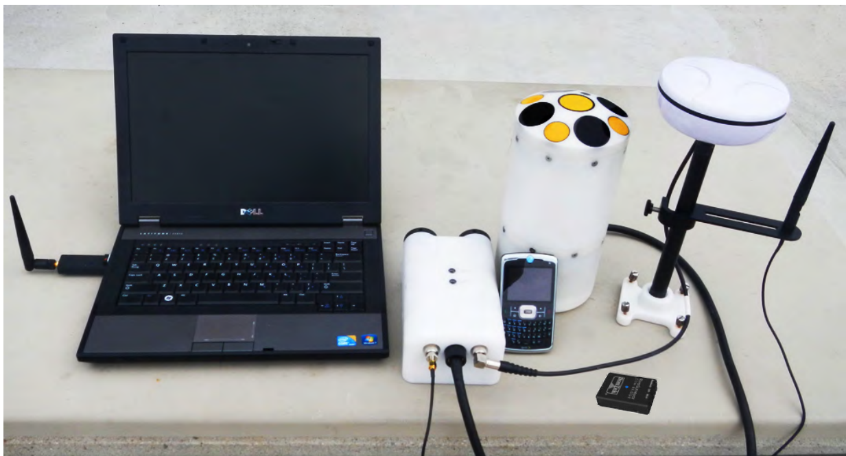
Figure 196. Configuration B – PCM DGPS. Figure shows the different methods of connecting to the PCM: Via mobile phone (through Bridge), or through PC (via radio dongle on the left of the image). Figure also shows the GPS antenna with accompanying radio antenna and extension cord.
