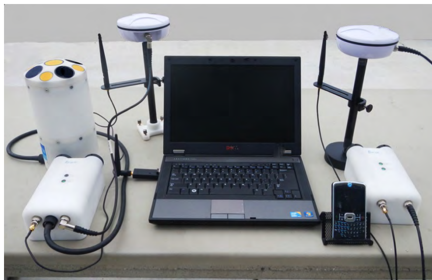
Figure 199. Configuration C – PCM RTK-GPS. Figure shows the different methods of connecting to the PCM: Via mobile phone (through Bridge (not pictured)), or through PC (via radio dongle on the left of the image). Figure also shows the GPS antenna with accompanying radio antenna and extension cord as well as the base station (typically mounted on a tripod as in the following figure).
