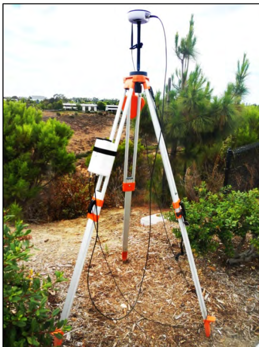
Figure 200. Base Station for Configuration C – PCM RTK-GPS. Figure shows a typical setup with GPS antenna on center of tripod and PCM attached to one of the tripod's legs via the provided adaptor bracket. Note PCM can be placed on ground as well.
