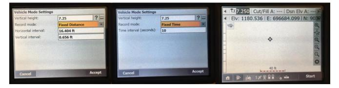
After the first measurement you will need to input the point number, point code, point type. I am not sure that surface is the best selection. I used it for this job but any point type will work. You will now see points being collected.
