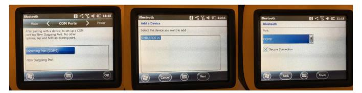
Make sure you confirm the comport and note it for use later (in this case Com8). I also have found that checking these two boxes during use of the sonar keeps the connection from dropping. This is found under the power tab at the top.
