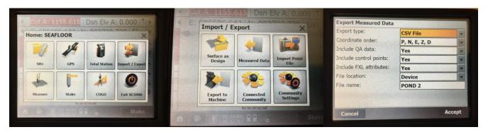
This file is stored in the output folder of this project. Can also copy the file onto a thumb drive.
