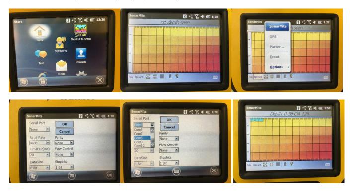
Your TSC3 should now be connected to your SonarMite. The BlueTooth light on the device should be solid blue. If your sounding unit is in water the power light should be green. Now start SCS900 by pressing the windows button on your data collector and picking the SCS900 icon. This is a picture of the version I am using. I also disable turning off the screen when performing a survey to make sure the bluetooth connection was not lost to the Sonarmite under the power options.
