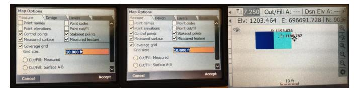
As you can see the current elevation of the GPS is different than the measured elevation displayed on the point (Elv is 1203.464 and the point elevation is 1193.636). This shows that we are getting combined data from the GPS and the sonar. Once the job is completed it is time to export the points so they can be imported into your software. Go to Import Export / Measured Data / CSV File. You can also export a DXF or other formats.
