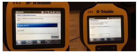
On the top of the screen choose COM Ports. Now select New Outgoing Port. Pick your device from the list. In this case it is SMIL50516. It will now assign a comport. In this case COM8. Uncheck the secure connection box.
