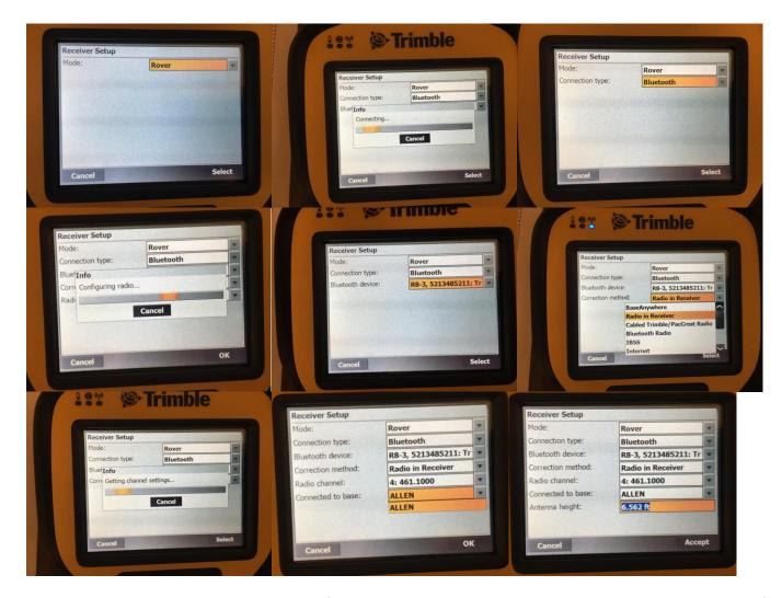
Antenna Height should be the height you use for checking control. Most companies use a 2 meter pole or 6.562 feet.
