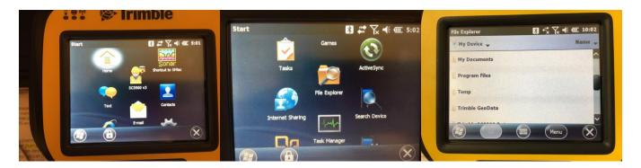
Next open the Trimble Folder, then the Trimble SCS900 folder. In this folder find the SMtsc file. I use the up and down arrows highlight the SMtsc file.
