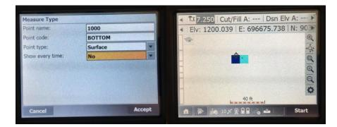
To check that you are getting readings from the sonar you will want to turn on point elevation display. If you press the gear in the lower right above the start button you will get this menu where you can turn on point elevation display.
